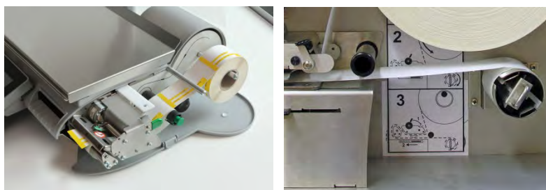
Figure 3-16: Labels Loaded in Stripped Mode – UC-CWx (left), UC-LP (right)
