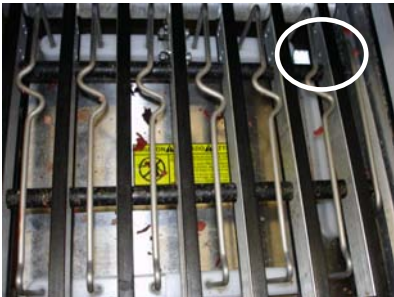
Clean the reflector on the scale platter. If it is dirty or covered with any debris, this can cause E65 or E66 errors.
