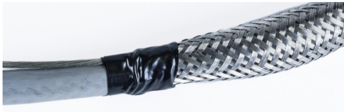
Figure 2-54: Outer Sheath Secured with Electrical tape
