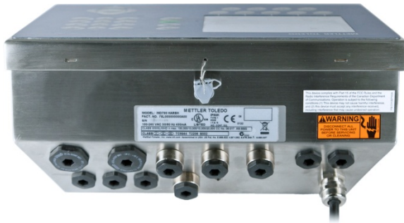
Figure 2-123: Harsh Enclosure, Sealing Complete
