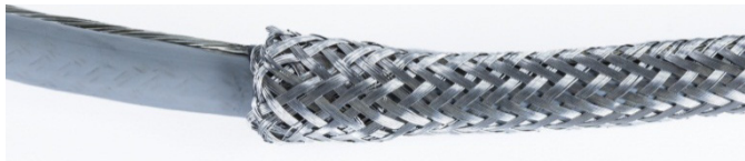
Figure 2-55: Outer Sheath Pushed Up Over Taped End
