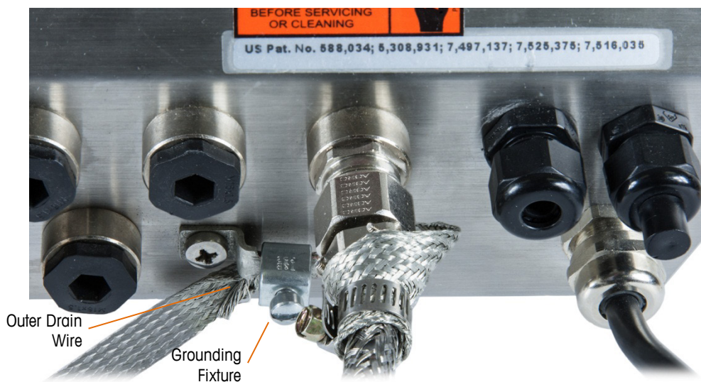
Figure 2-65: Cable and Strap Assembly Installed on Harsh Enclosure
