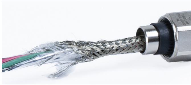
Figure 2-59: Inner Sheath Frayed
