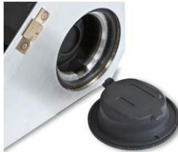
Remove the cover by pulling it out of the terminal. Note the tabs on the battery cover.
