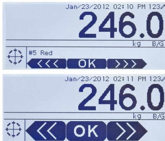
**Figure 4-7: Composite SmartTrac Graphic Display: Small (top) and large (bottom)**
