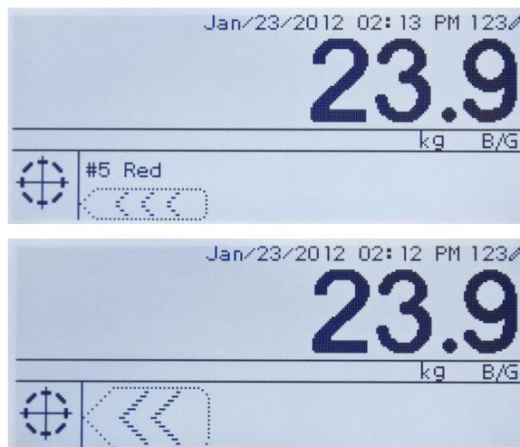
**Figure 4-8: SmartTrac Graphic Display, Zones Not Activated: Small (top) and large (bottom)**
