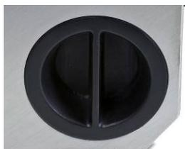
Install the battery cover by aligning its tabs with the slots inside the battery cavity – the handle will be vertical. When it is fully inserted, the cover should be flush with the outside of the terminal.
