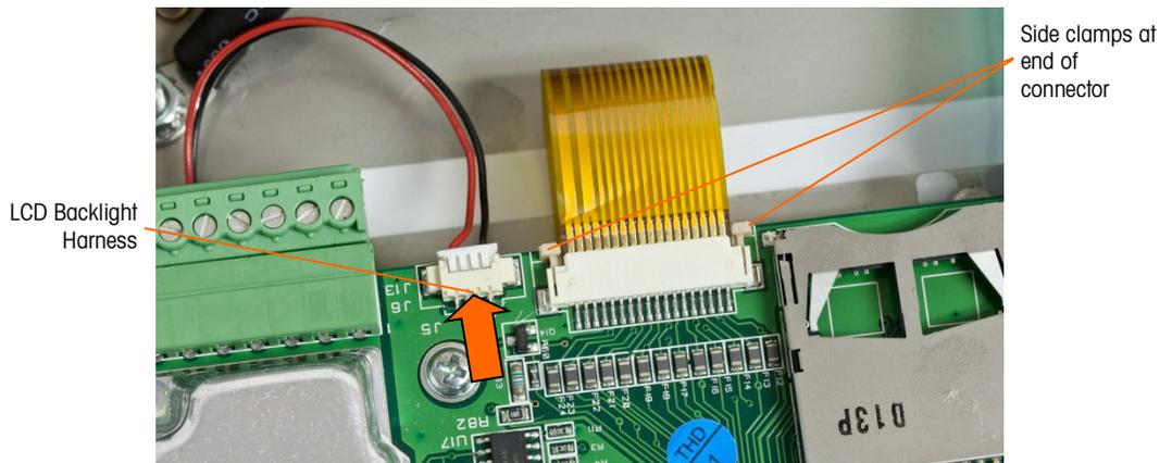
**Figure 5-12: Display Harness Removal**
