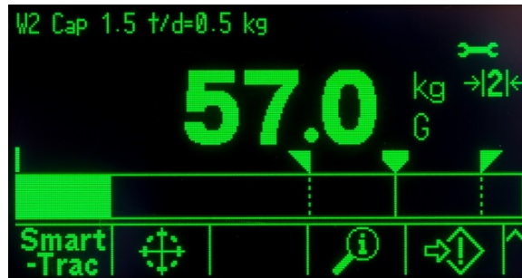
Figure 1-11: Small Material Transfer SmartTrac Enabled
