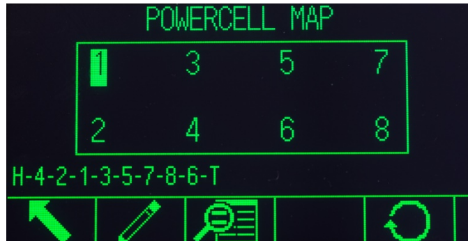
Figure 3-34: Completed POWERCELL Load Cell Map
