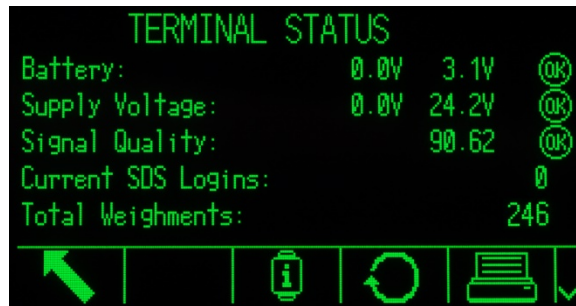
Figure 4-11: Terminal Status Screen with Load Cell and Reset Icons
